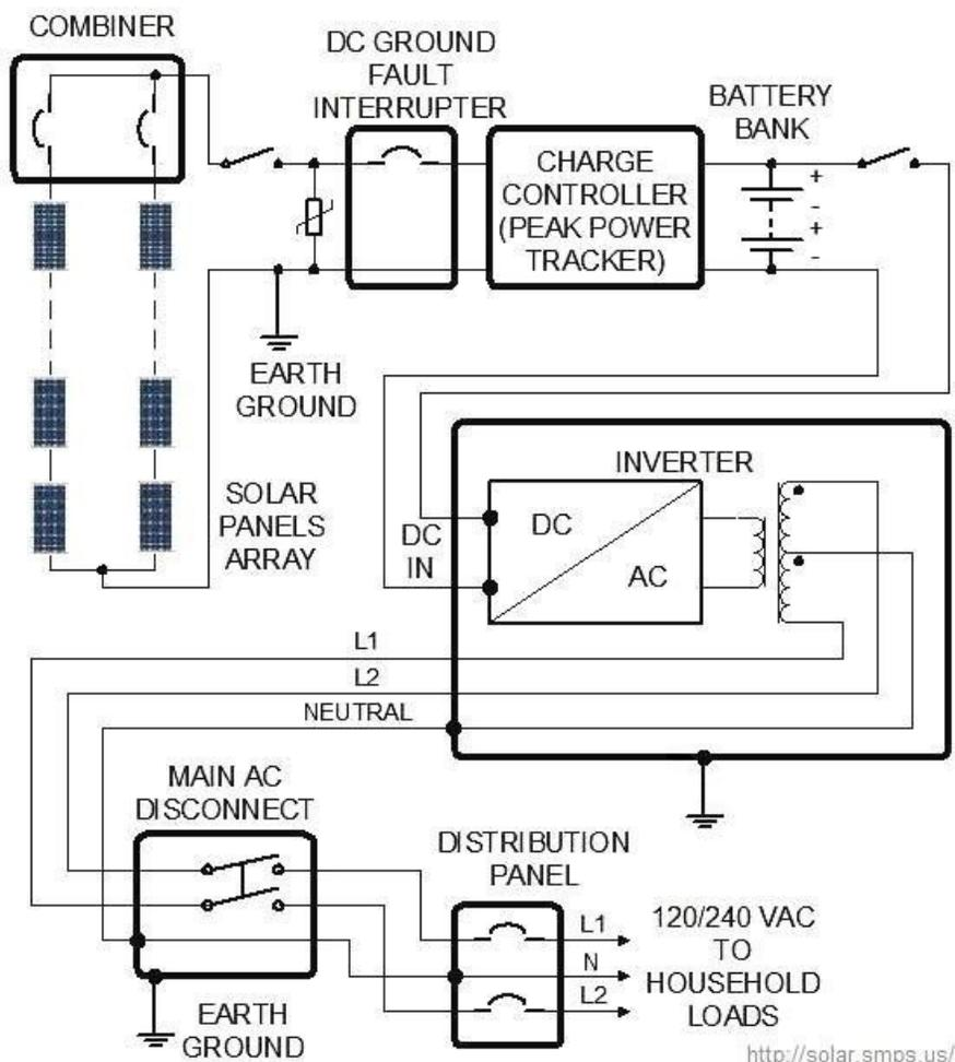
Particularly, one AC output conductor has to be grounded. In a single-phase 3-wire setup it has to be the neutral buss. PV panels can be connected in series and parallel- see various solar panel wiring methods. If you parallel several strings of solar panels, it is desirable to use a **combiner** with a fuse or a circuit
