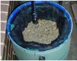
The filter described and illustrated in the paragraph above is a fast sand filter. Water passes quickly through the filter and small particles are removed. The sand in the filter needs to be washed quite regularly to remove accumulated particles from between the grains of sand.
