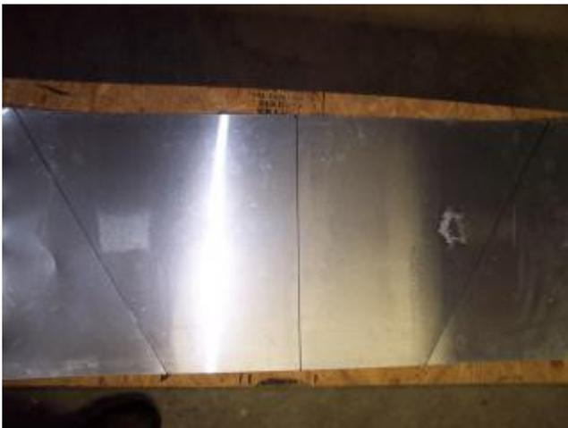
Step 1. Cut a piece of 14"-16" wide aluminum flashing to a length of just over 30".
