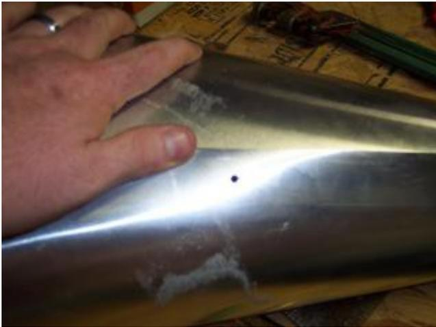
Step 8. Roll the metal up so that the marked side is overlapped to the line and clamp it. Drill a hole in the overlapping portion near the top, middle and bottom of the cone. Put a rivet in the hole from the INSIDE. The head of the rivet will be on the inside and is smooth. This way there is nothing for the bird to get snagged or cut on inside the cone.
