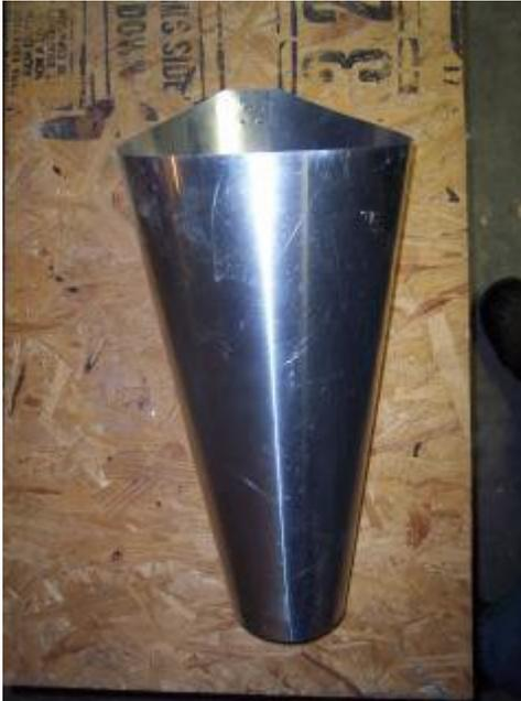
I decided that my first post should be informative. Here are instructions for building your own killing cones for broiler sized (4-8 lbs.) chickens. The final dimensions are 9" top opening, 4" bottom opening and a length corresponding to the width of flashing you use.
