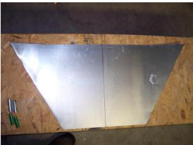
Step 6. Score the diagonal lines with a utility knife and fold gently away from the cut to tear the waste pieces off.
