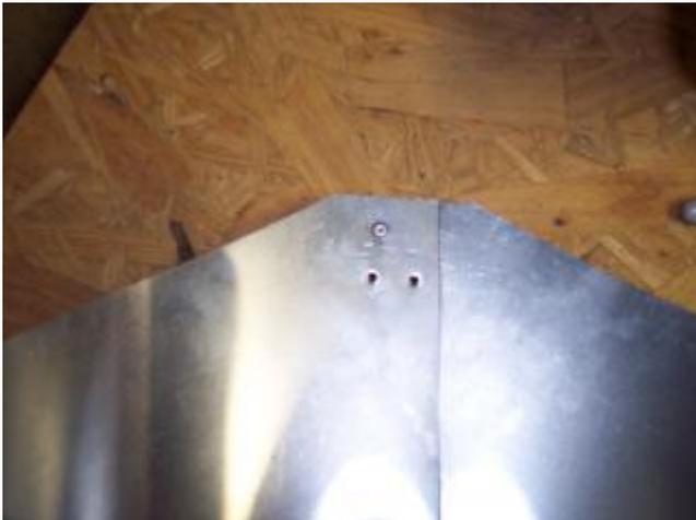
Step 9. Drill one or two holes near the top of the cone to hang it by.
