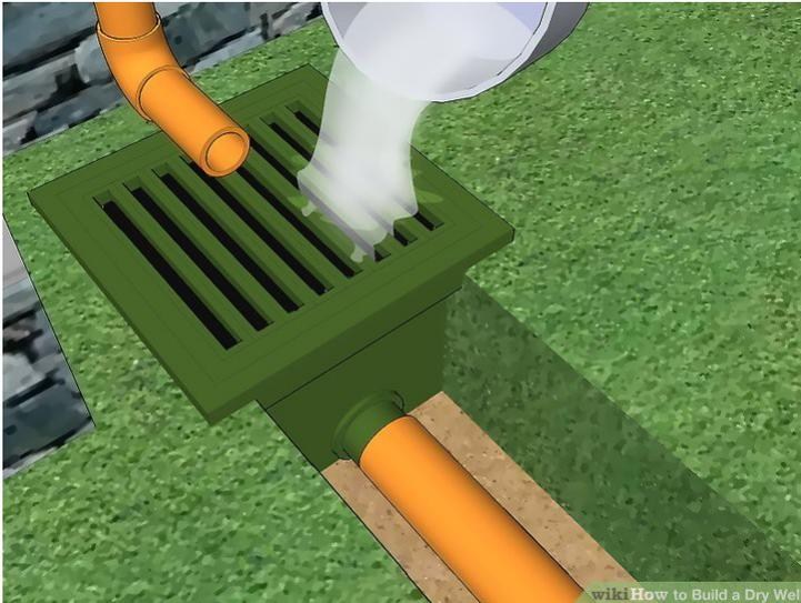
10. Pour water at the top of the pipe to verify that the water runs down into the holding tank.
