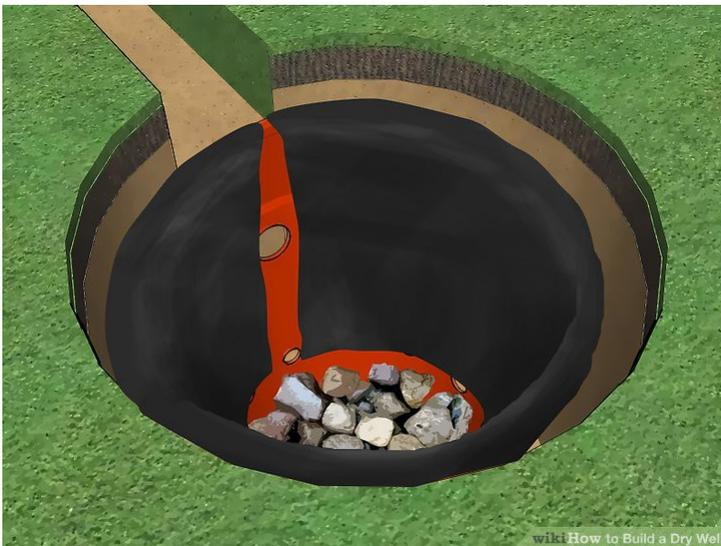
7. Place 6 inches (15.2 cm) of rock in the bottom of the holding container and line the interior of the holding container with landscape fabric.
