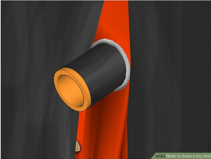
9. Wrap the end of the entry pipe in landscape fabric and insert end of perforated PVC pipe into entry hole in holding container. Caulk the pipe entry point and allow to dry for 1 hour.
