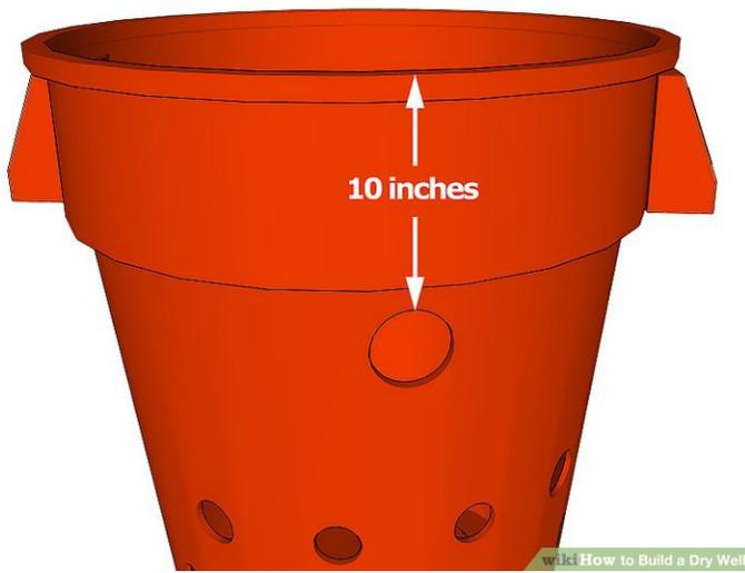
6. Cut an entry hole in the side of the holding container approximately 10 inches (25.4 cm) below the top of the container.
