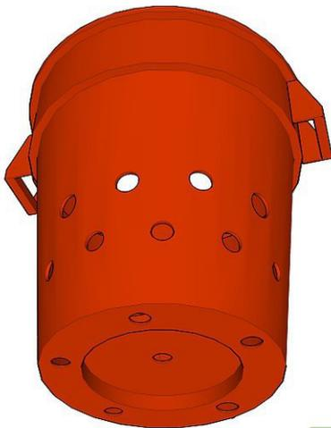
5. Drill 25 to 30 drainage holes along the bottom and halfway up the sides of the holding container.
