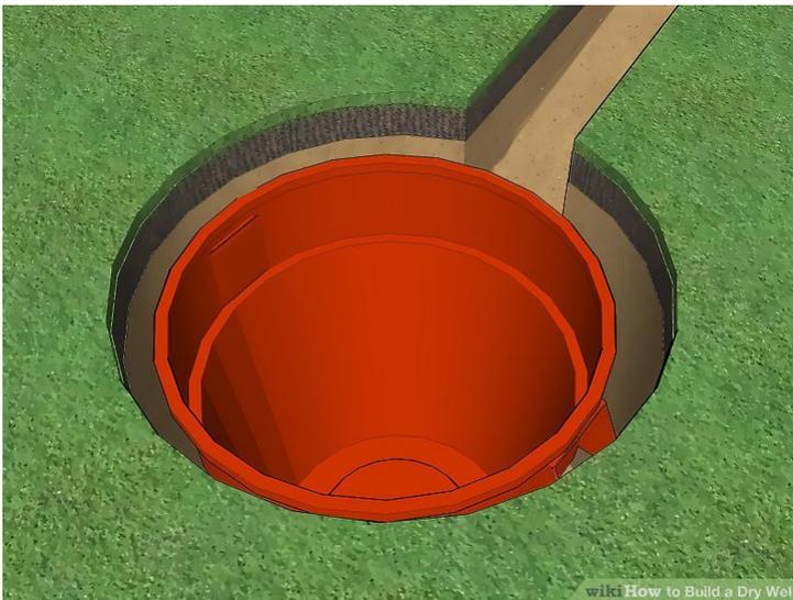
4. Sink the holding container into the holding tank pit.
