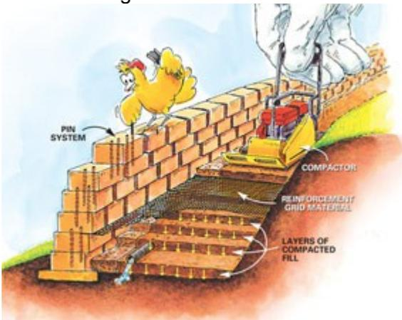
Compacted soil combined with a reinforced grid puts less pressure on the wall.
