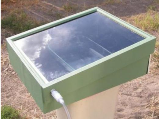
The author's solar still, with one pan in it. The still actually has room for two of these. Note that the glass top is at an angle, allowing the water to flow down to the catch tube.
