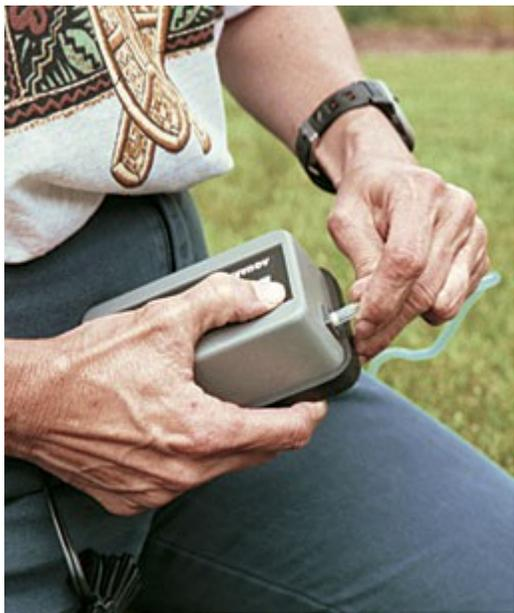
1. Attach one end of a piece of tubing to the pump; the other end will connect to the gang valve.
