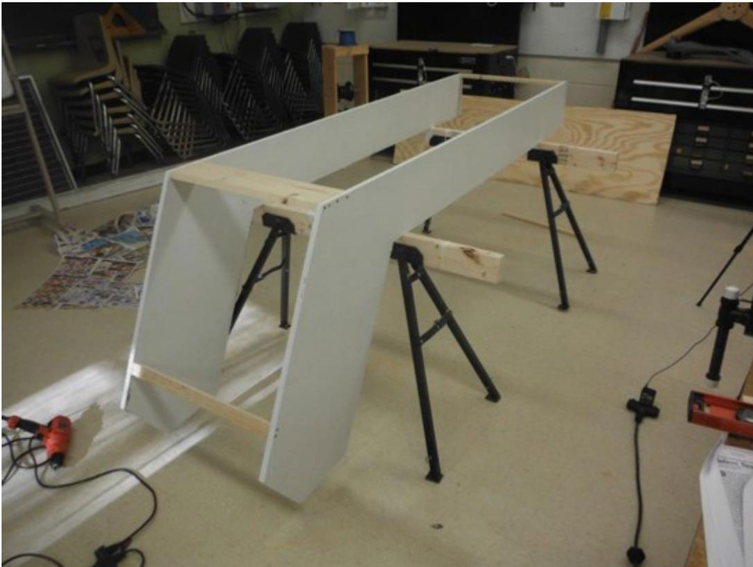
Before beginning assembly, you'll need to cut some braces to support the components of the solar dehydrator on the interior. Most of these braces will serve more than one function so it's important to use the correct one at each location. See the detailed drawing ("How it Works," above) for proper sizing and placement of the braces.
