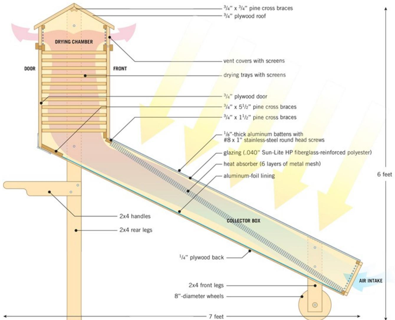
As you can see in the detailed drawing, the design includes a long, angled wooden box covered with clear plastic glazing and an open bottom end for air intake. Inside, the box holds diagonal layers of black metal screen. The vertical drying chamber on top has a back door to access food-drying trays inside.
