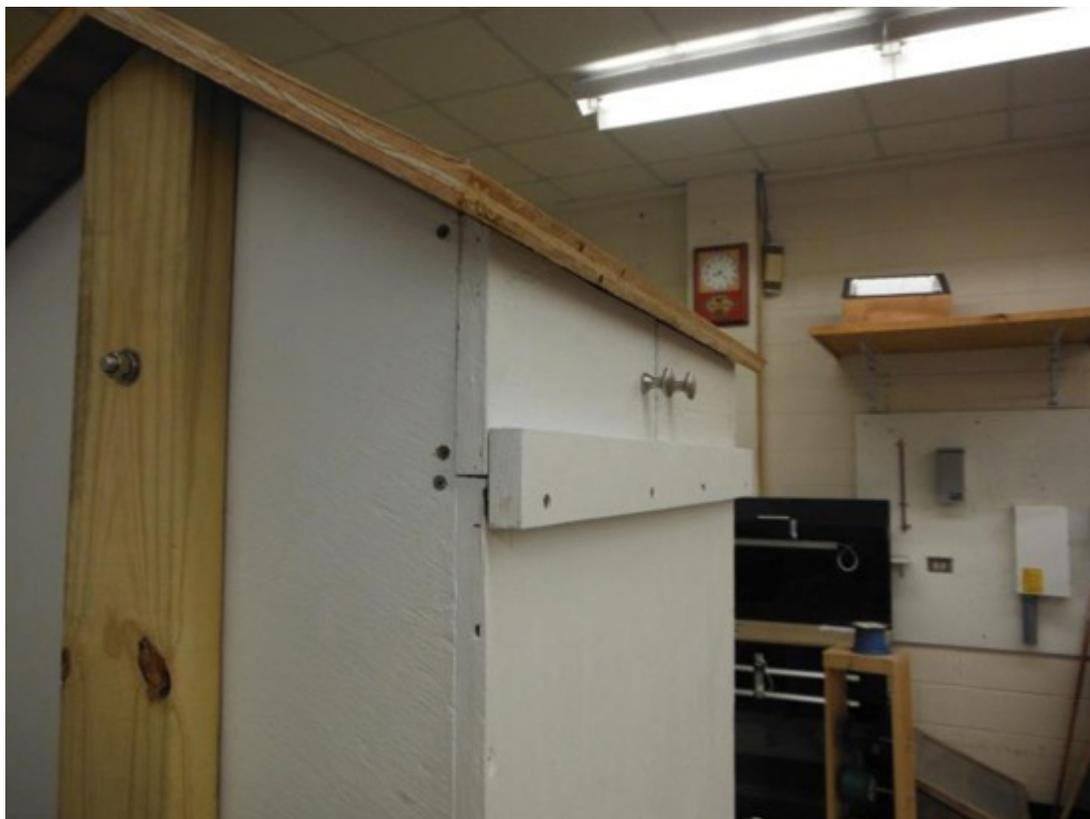
This dehydrator design calls for vents at the top of the drying chamber on both the front and back, just below the roof. These vents are essential for effective operation of the food dryer: As cool air enters the intake at the bottom and become heated in the collection chamber, it must rise into the drying chamber where it will absorb moisture from the food before exiting through the upper vents.
