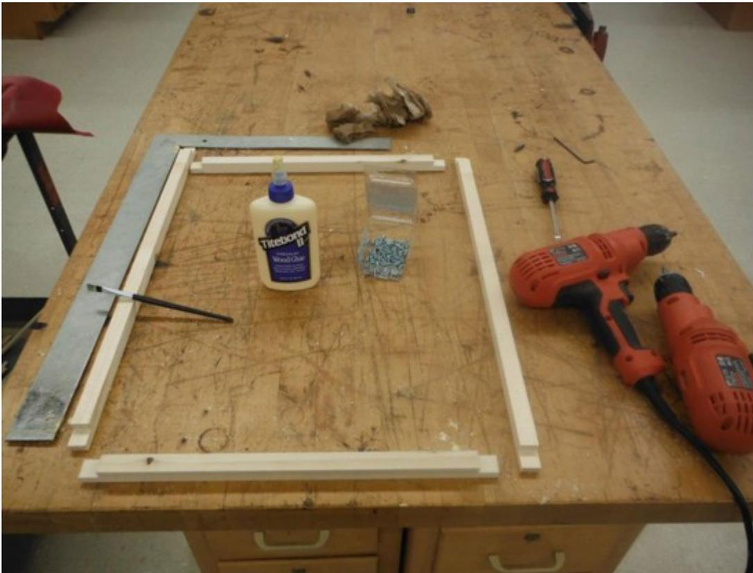
The drying chamber will hold 11 rectangular trays for dehydrating food. You'll want to build trays with wooden frames that will stand up to lots of use, but with screened bottoms so air can circulate around the drying food. Use four 1-by-6s to make the frame components. Cut two of these boards into 22-1/4-inch lengths, and the other two into pieces measuring 16 inches long.
