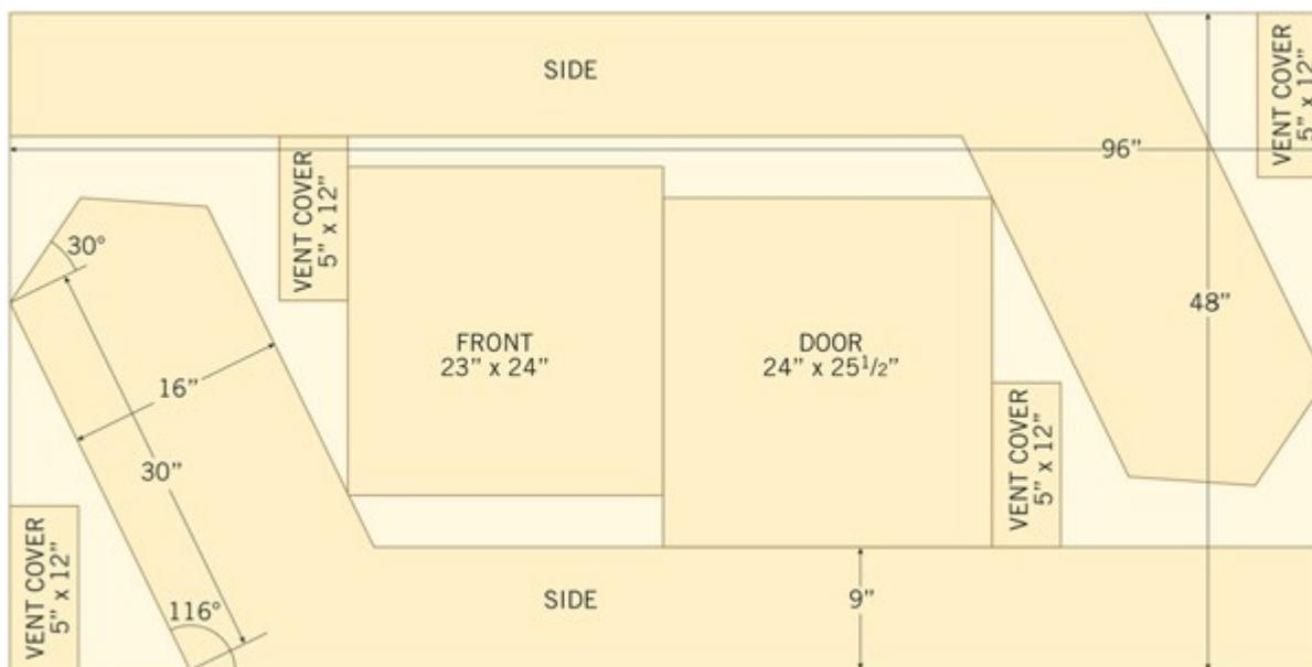
Most of the wood required for these solar food dehydrator plans can be cut from a single 4-by-8-foot sheet of three-quarters-inch-thick exterior-grade plywood. Measure and mark the plywood using the cutting diagram (above) as your guide. Note that the dryer sides are cut in a single piece so there's no joint between the collector box and the drying chamber. You should mark the dehydrator's sides on opposite edges of the plywood sheet to leave space in the center for the other pieces you'll need.
