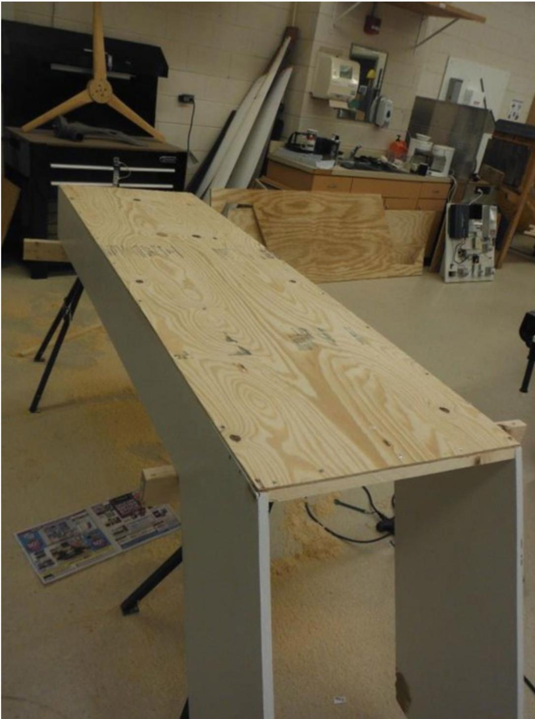
Remember that sheet of quarter-inch exterior grade plywood in the materials list? Cut a 24-inch-wide piece from it that's the same length as the bottom of the collector box. In this design, the length is 6 feet and 11 inches, but the dimension will be different if you changed the angle of the collector to make a solar dehydrator specific to your latitude.
